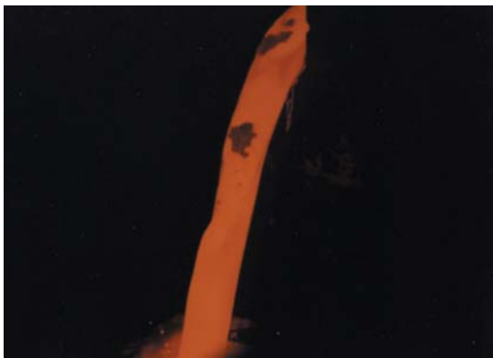
Fig. 3 — A pour stream showing turbulence, solid inclusions, and streamlines of material that are either lower temperature or lower emissivity than their surroundings.
